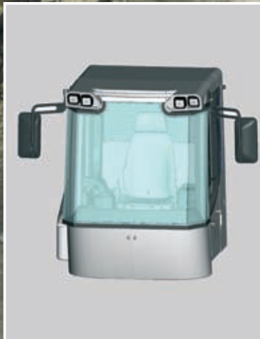
Cab with laminated safety glass
