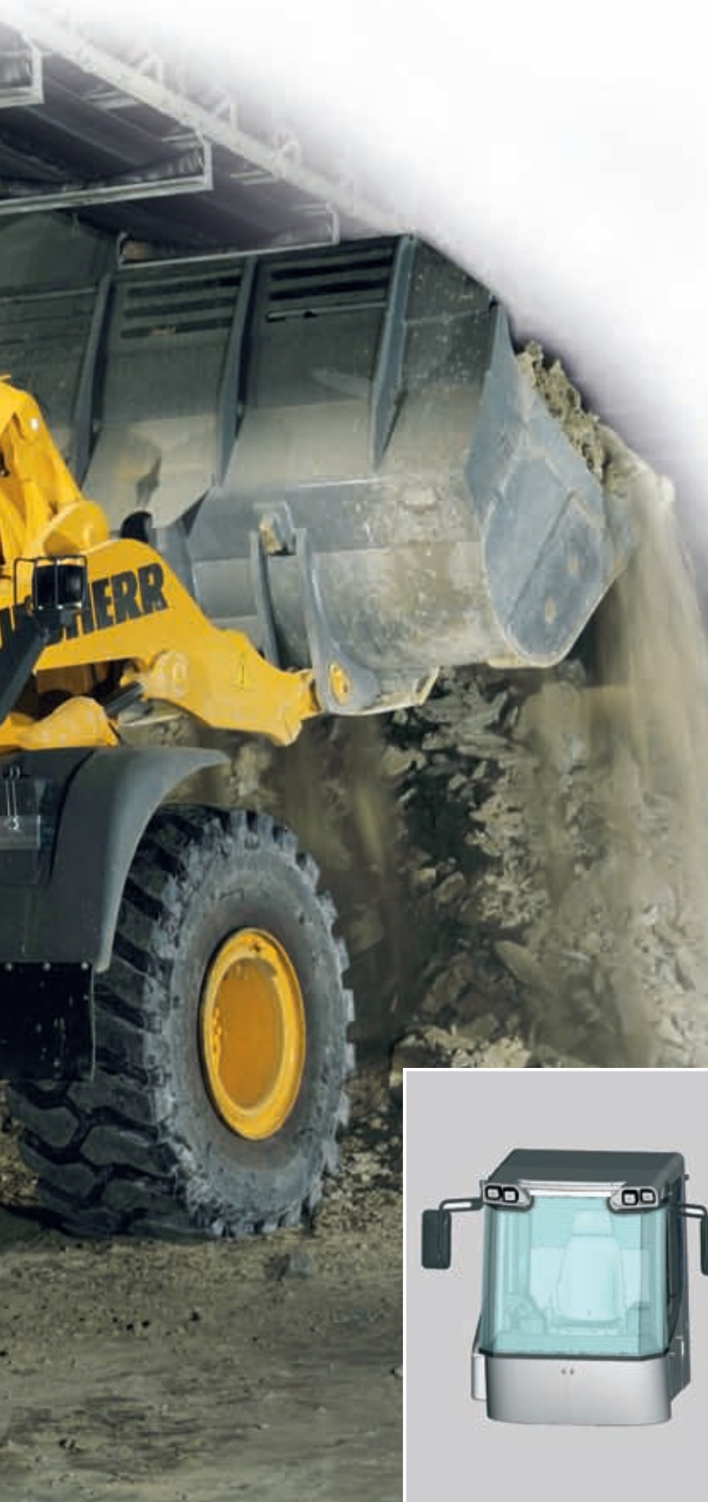
Cab with laminated safety glass
