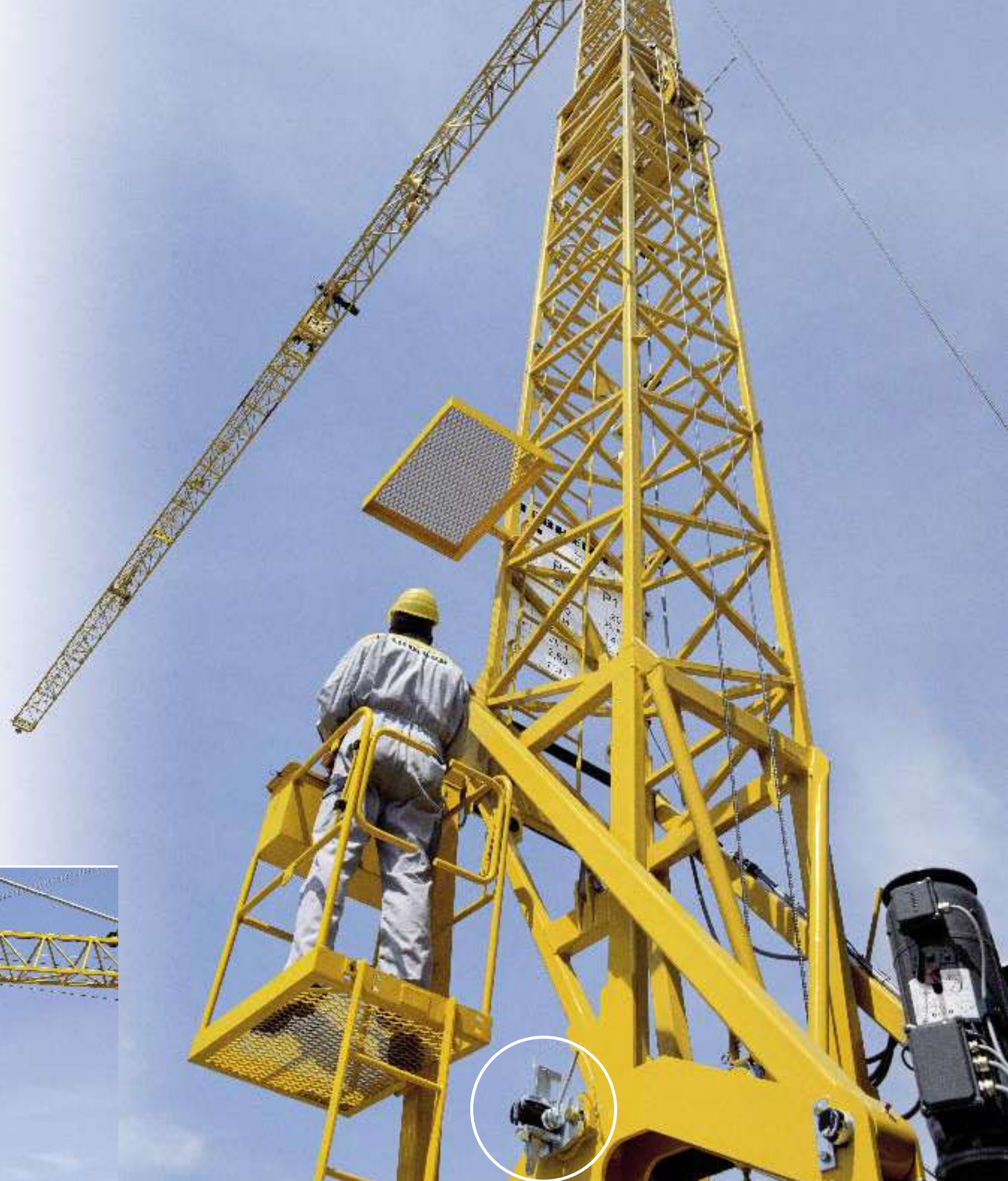
The Quick Connection system for rapid tower locking.
