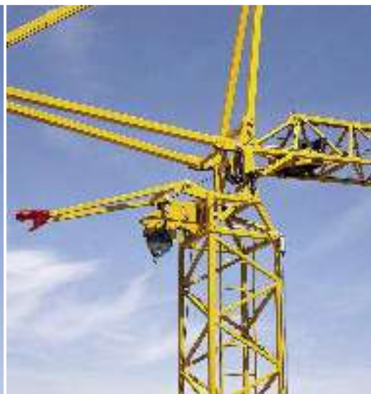
Central jib pivoting ensures uniform distribution of forces in the tower.
