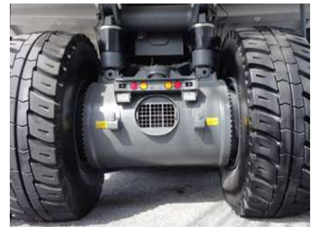
Service door on axle box for inspections
