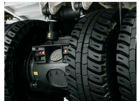
Service door on axle box for inspections
