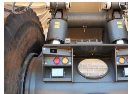
Service door on axle box for inspections
